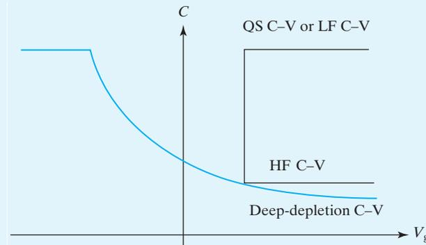
FIGURE 5–29 Deep-depletion C–V.
