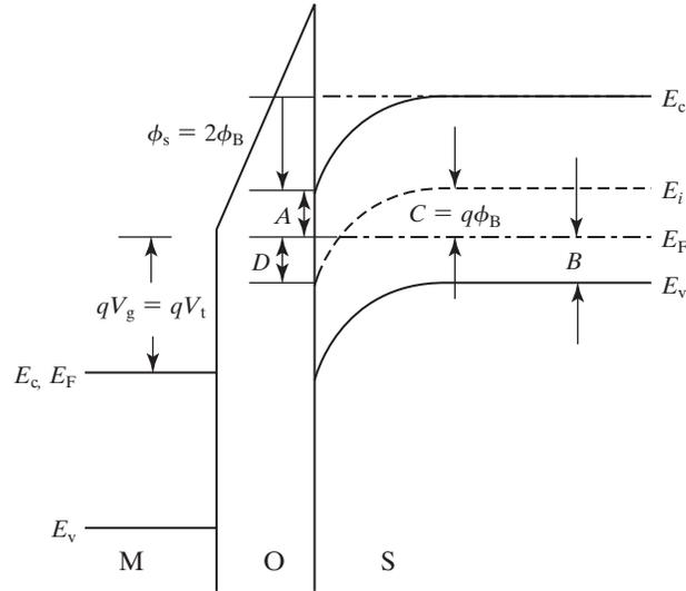
**FIGURE 5-7** The threshold condition is reached when  $n_s = N_a$ , or equivalently,  $A = B$ , or  $\phi_s = \phi_{st} = 2\phi_B$ . Note that positive  $\phi_{st}$  corresponds to downward band bending.
