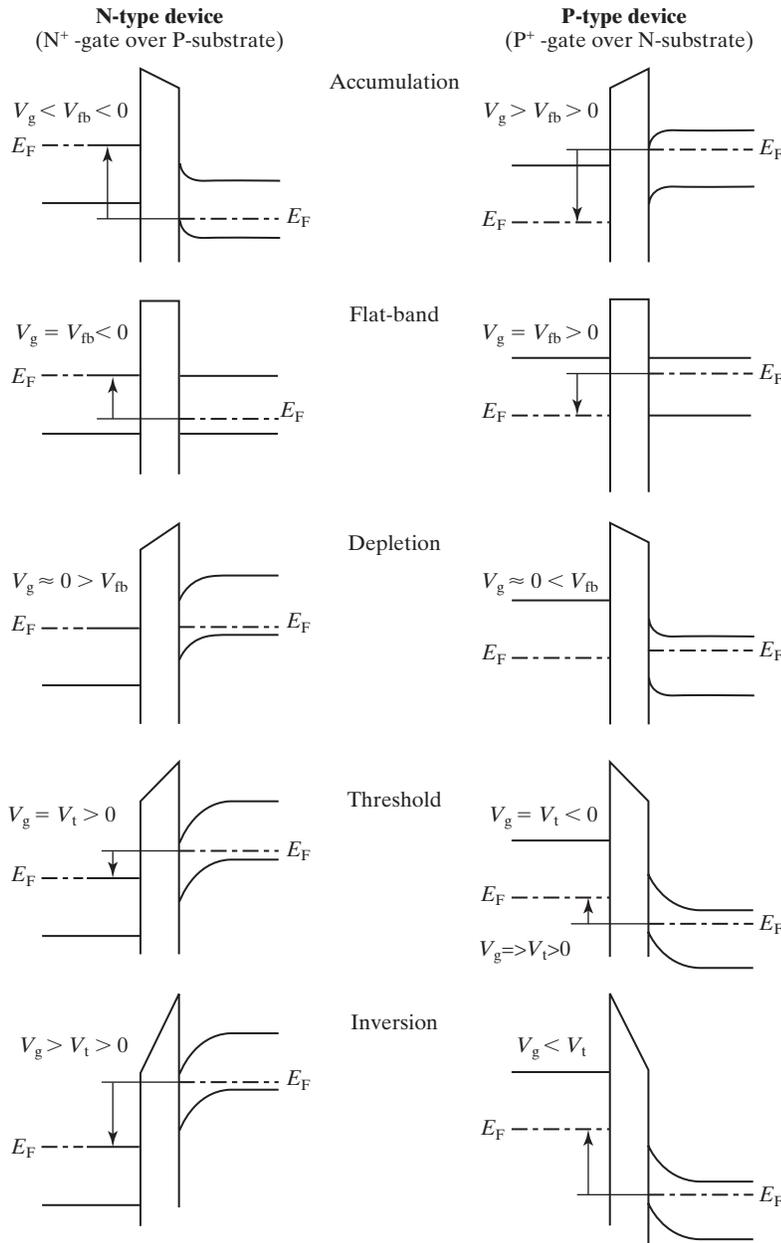
**FIGURE 5-33** Energy band diagrams of the two dominant types of MOS capacitors. An N-type device is so named because it has N-type inversion charge that increases with a more positive  $V_g$ , and a P-type device has P-type inversion charge increasing with a more negative  $V_g$ .
