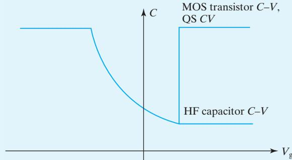
**FIGURE 5-19** C-V curves of MOS capacitor and transistor.
