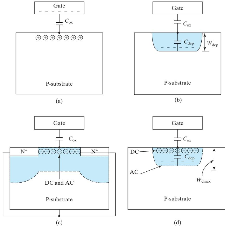
**FIGURE 5-17** Illustration of the MOS capacitor in all bias regions with the depletion-layers shaded. (a) Accumulation region; (b) depletion region; (c) inversion region with efficient supply of inversion electrons from the N region corresponding to the transistor  $C-V$  or the quasi-static  $C-V$ ; and (d) inversion region with no supply of inversion electrons (or weak supply by thermal generation) corresponding to the high-frequency capacitor  $C-V$  case.
