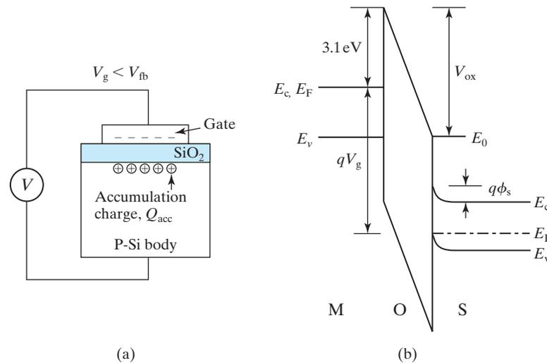
**FIGURE 5-5** This MOS capacitor is biased into surface accumulation ( $p_s > p_0 = N_a$ ). (a) Types of charge present.  $\oplus$  represents holes and  $-$  represents negative charge. (b) Energy band diagram.
