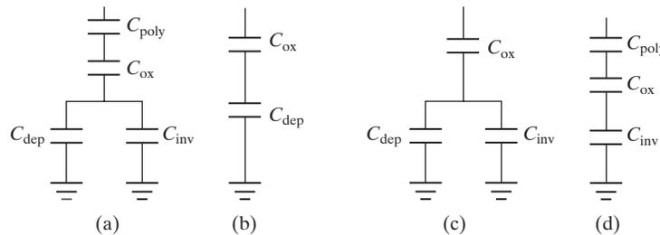
**FIGURE 5-27** Equivalent circuit for understanding the  $C$ - $V$  curve in the depletion region and the inversion region. (a) General case for both depletion and inversion regions; (b) in the depletion regions; (c)  $V_g \approx V_t$ ; and (d) strong inversion.
