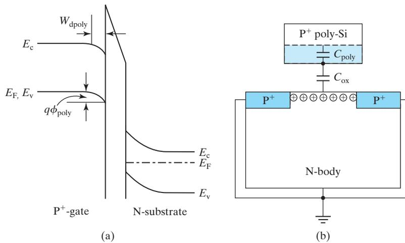
**FIGURE 5-23** Poly-gate depletion effect illustrated with (a) the band diagram and (b) series capacitors representation. An N<sup>+</sup> poly-Si gate can also be depleted.
