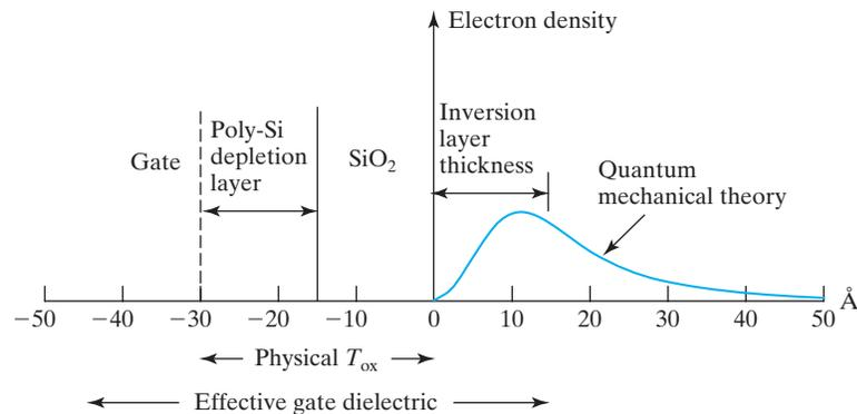
**FIGURE 5-24** Average location of the inversion-layer electrons is about 15 Å below the Si-SiO<sub>2</sub> interface. Poly-Si gate depletion is also shown.
