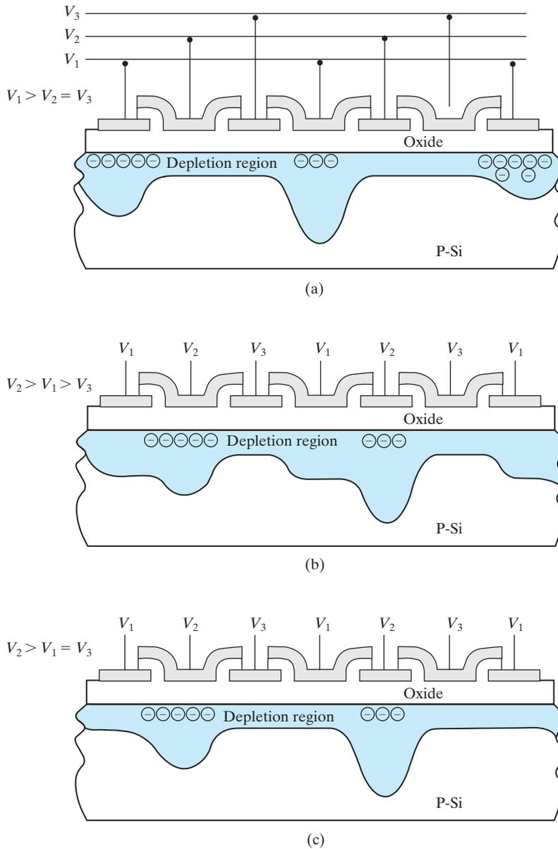
**FIGURE 5-30** How CCD shifts the charge packets. The array is biased in the sequence (a), (b), (c), (a), (b), (c), (a) ... . The drawing in (c) is identical to (a) but with all the charge packets shifted to the right by one capacitor element.
