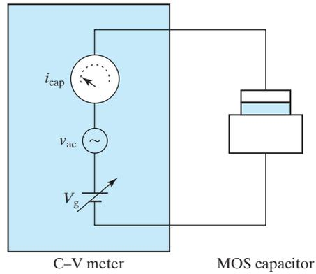
FIGURE 5-15 Setup for the C-V measurement.
