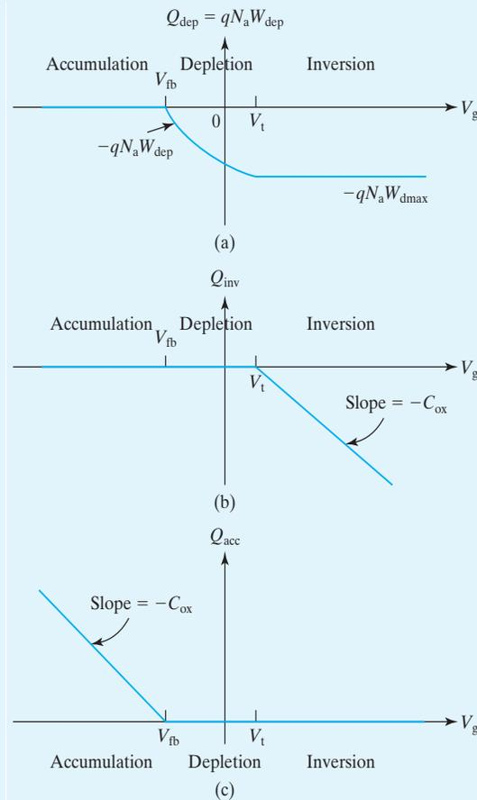
FIGURE 5–13 Components of charge ( $C/cm^2$ ) in the MOS capacitor substrate: (a) depletion-layer charge; (b) inversion-layer charge; and (c) accumulation-layer charge.
