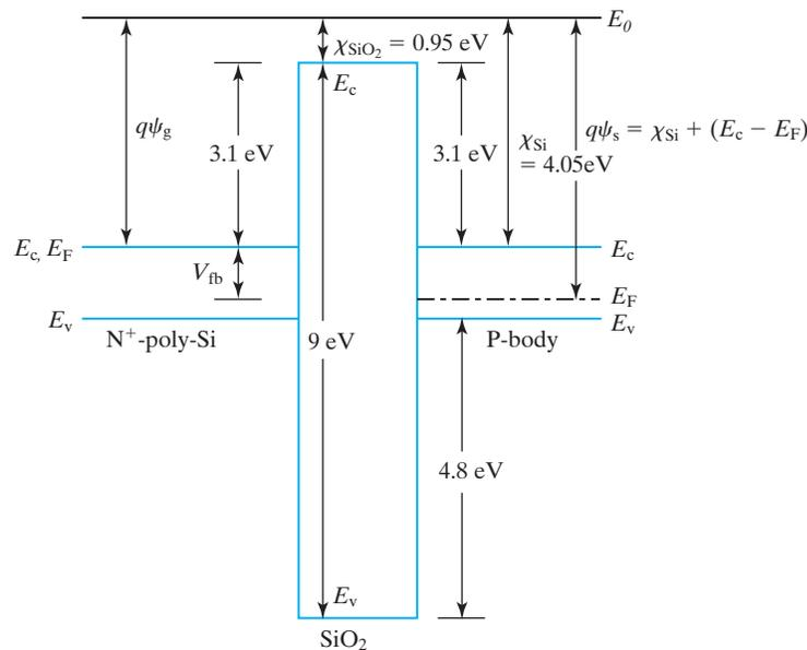
**FIGURE 5-4** Energy band diagram of the MOS system at the flat-band condition. A voltage equal to  $V_{\text{fb}}$  is applied between the N<sup>+</sup>-poly-Si gate and the P-silicon body to achieve this condition.  $\psi_g$  is the gate-material work function, and  $\psi_s$  is the semiconductor work function.  $E_0$  is the vacuum level.
