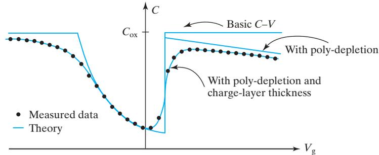
**FIGURE 5-26** The effects of poly-depletion and charge-layer thickness on the  $C$ - $V$  curve of an  $N^+$  poly-gate, P-substrate device.
