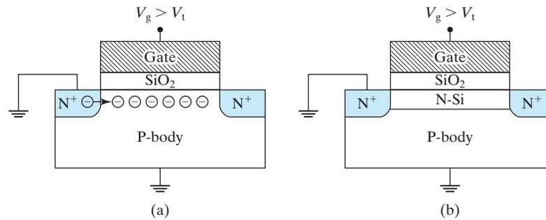
**FIGURE 5-10** (a) The surface inversion behavior is best studied with a PN junction butting the MOS capacitor to supply the inversion charge. (b) The inversion layer may be thought of as a thin N-type layer.
