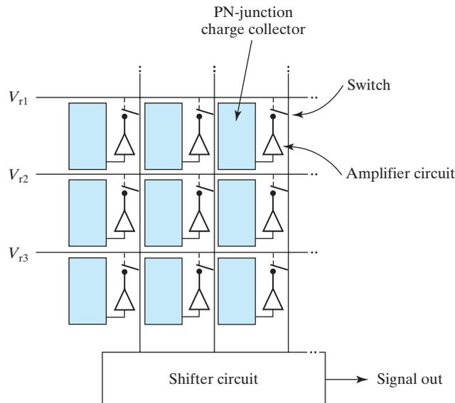
**FIGURE 5-32** Architecture of a CMOS imager. Each array element has its own charge-to-voltage converter represented by the triangle. Actual imagers may support hundreds to over a thousand rows and columns of pixels.
